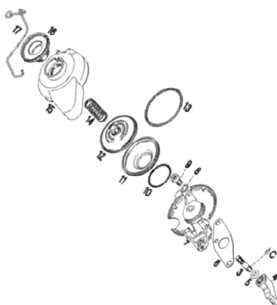
Version 1, pneumatic timed exhaust valve.
